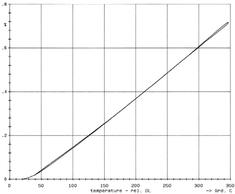
Fig. 8. Relative elongation as a function of temperature for the new composite material during heating and cooling with the very small elongation differences between cooling and heating
