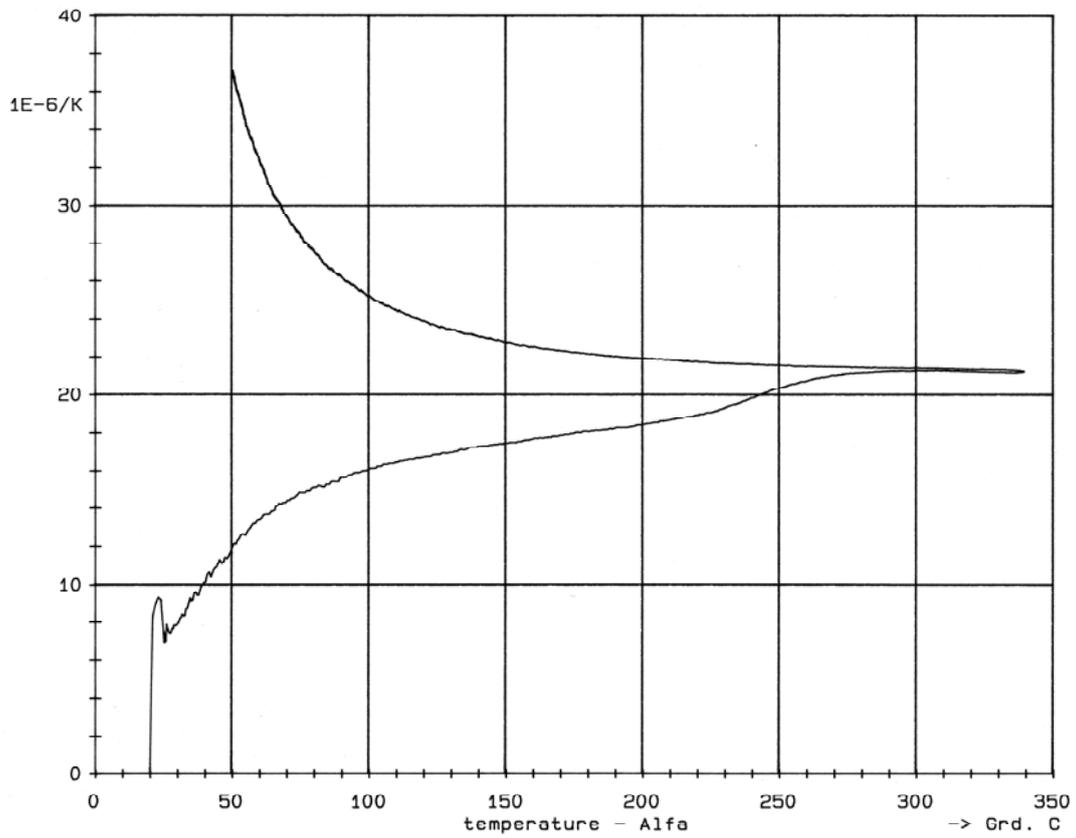
Fig. 1. Coefficient of linear expansion  $\alpha$  for the AlSi standard alloy in a raw state during heating and cooling
