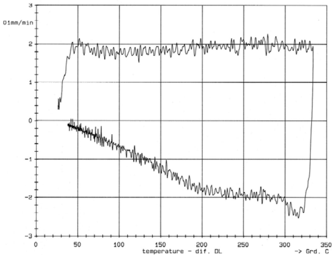
Fig. 10. Course of derivative of specimen dimension increase to the time as a function of temperature ( $T$ ) during heating and cooling without phase transition during heating and cooling with the very small elongation differences between cooling and heating
