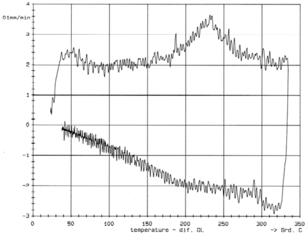
Fig. 9. The course of derivative of specimen dimension increase to the time as a function of temperature ( $T$ ) during
