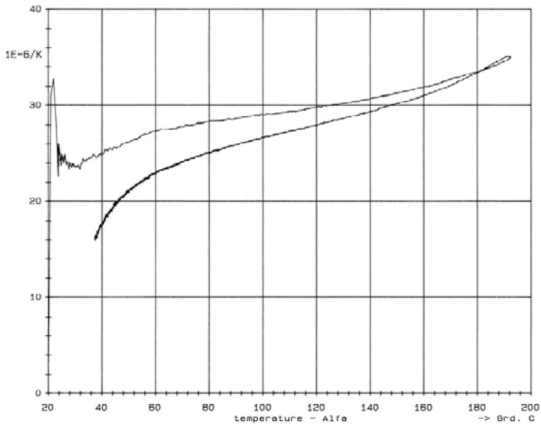
Fig. 4. Coefficient of linear expansion  $\alpha$  for the AlSi alloy during heating and cooling with the  $\alpha$  positive and negative differences between cooling and heating
