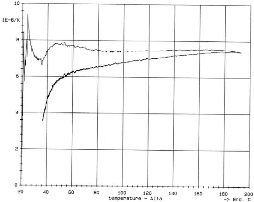
Fig. 3. Coefficient of linear expansion  $\alpha$  for the AlSi alloy during heating and cooling with the  $\alpha$  negative differences between cooling and heating
