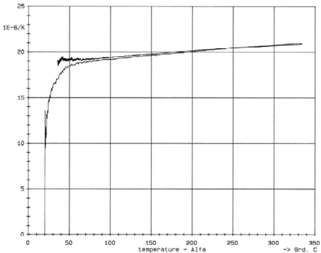
Fig. 6. Coefficient of linear expansion  $\alpha$  for the AlSi alloy during heating and cooling with the very small  $\alpha$  differences between cooling and heating
