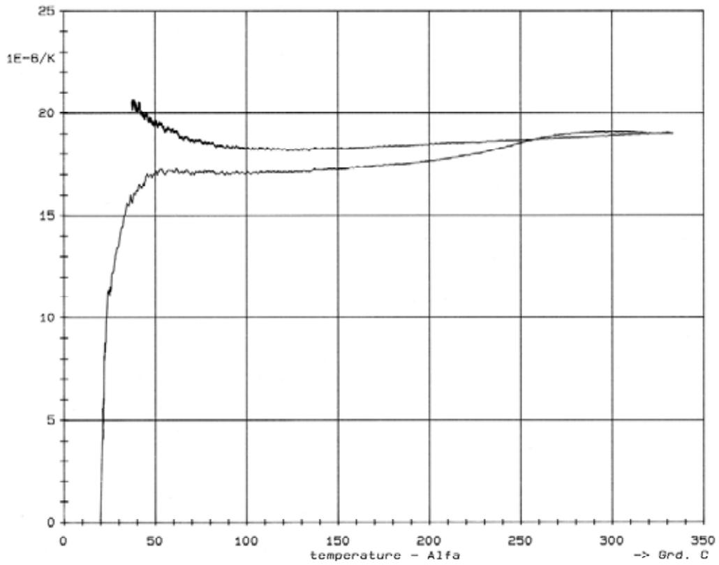
Fig. 5. Coefficient of linear expansion  $\alpha$  for the AlSi alloy during heating and cooling with the a positive, negative and positive differences between cooling and heating
