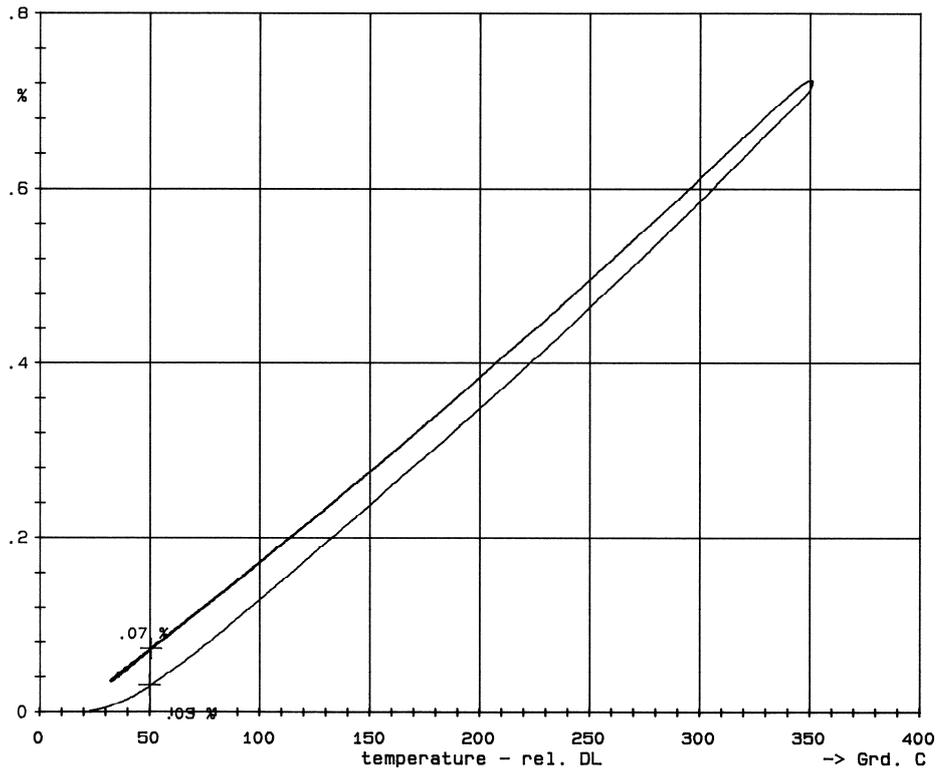
Fig. 7. Relative elongation as a function of temperature for the new composite material during heating and cooling with the positive elongation differences between cooling and heating
