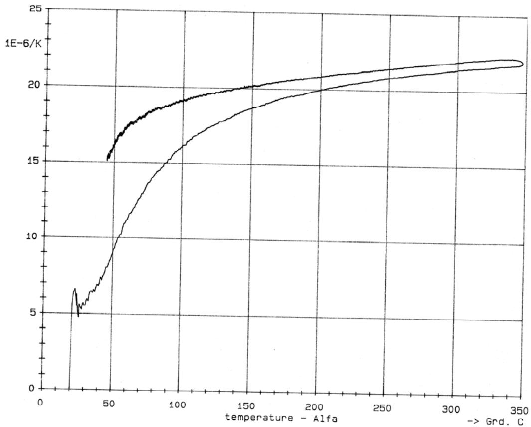
Fig. 2. Coefficient of linear expansion  $\alpha$  for the AlSi alloy during heating and cooling with the  $\alpha$  positive differences between cooling and heating
